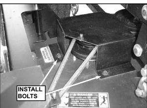
**STEP 8:** Lay supplied pulley guard onto deck, aligning holes in guard with holes in deck. Install with bolts securing original guard, tightening securely.
